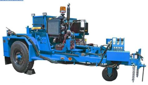
The Reel Trailer is equipped with a standard gasoline engine and offers a load capacity of 14,000 lbs. It comes with a powered hydraulic reel lift and a centralized control station. The trailer features electric brakes, a safety break-away system, ICC lights, and customizable design options.
