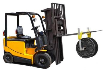
The Forklift Reel Loader is a specialized tool designed to transport reels up to 96 inches in diameter and weigh up to 10,000 lbs. It easily attaches to forklift forks with a "T" handle bolt and
