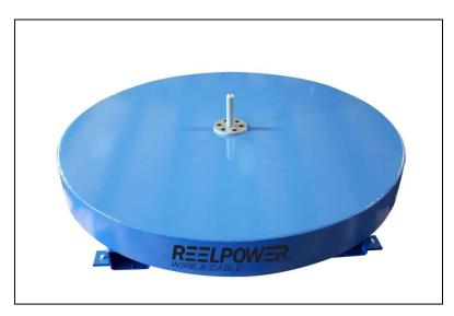
This unit is a manual payoff which can also be powered. When powering it, we typically pair it up with a simple dancer mechanism to control the speed only. This payoff is usually used when there are bad or broken wooden reels with product on them, the user can place the wooden reel on the BRT and pay off the material, even if the wooden reel is broken.
