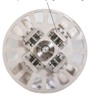
Manually adjustable back plate for varying coil widths
