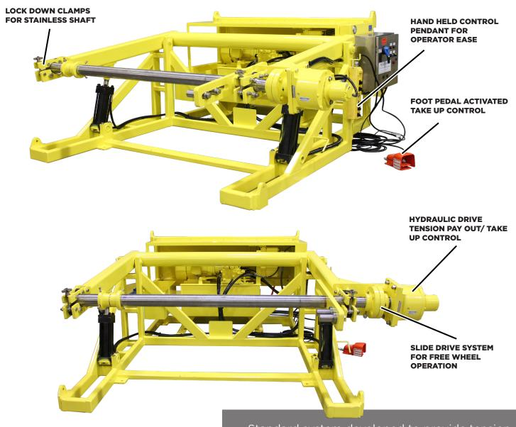
Standard system developed to provide tension controlled pay out and take up operations. Capable of 1,000 lbs of line tension at a 42 inch radius and line speeds of 50 feet per minute base on a 48 inch drum diameter. Custom systems built for your application.
