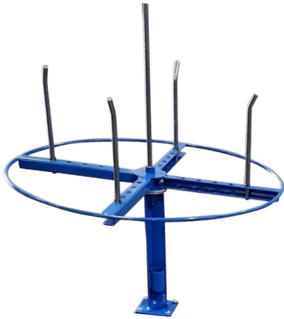
TURNTABLE 24" Diameter With adjustable ID pins PN 14000-37
