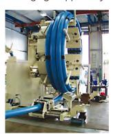
to unload the finished coil. Automatic pipe layering and auto stop at pipe end are standard across the range.
