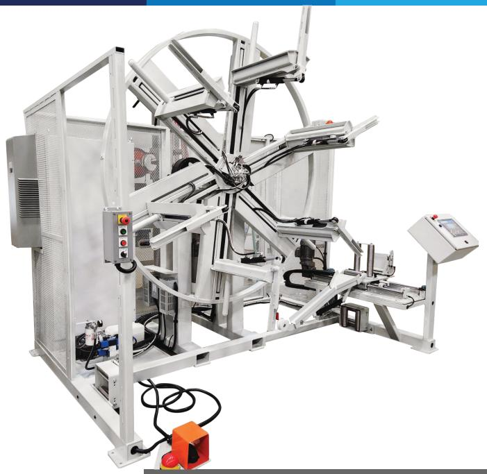
Standard 480V/3PH/60Hz power supply and 90 psi air supply is required unless other is specified.
