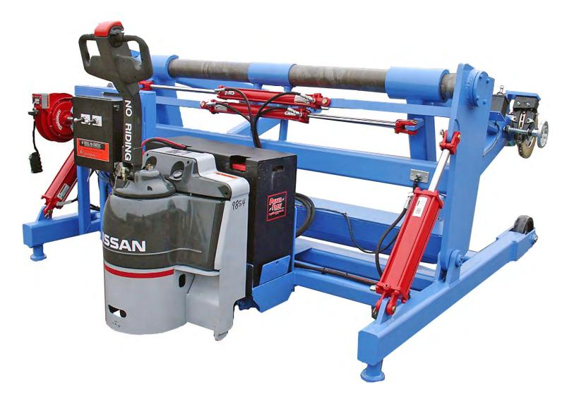
Standard Capacity 96" diameter 60" wide x 13,000 lb. Load Capacity.
