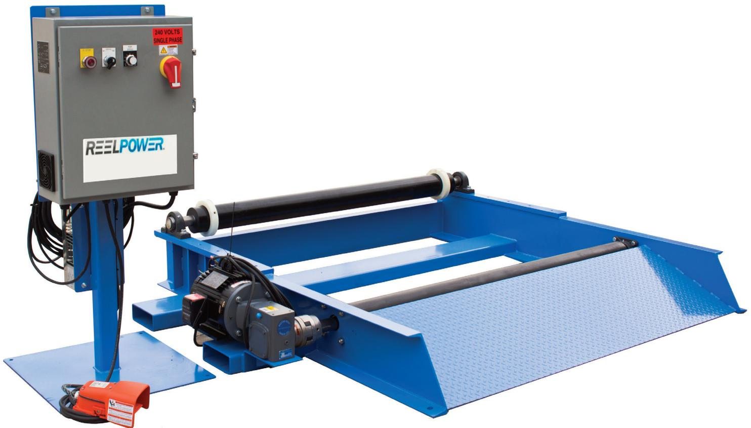
Shown above is our PRR10 with a Pedestal Mounted controls and Variable Speed Operator Controlled Footswitch.
