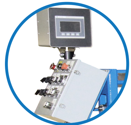
INTEGRALLY MOUNTED CONTROL PANEL
