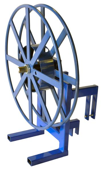
Custom Adaptors for existing Combo Units for mounting a single compartment paralleling reel. Includes heavy duty drop-in bracket with fixed 2" dia. stub shaft and reel 2 1/8" locking collars. RPR 15 Single compartment paralleling reel, 40" O.D. x 16" I.D. x 8" wide.
