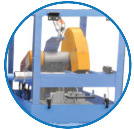
INTEGRATED HEAVY DUTY AUTOMATIC CHOP SAW
