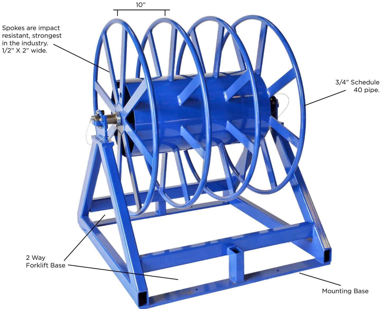
**Standard Combo Paralleling Cable Reel Stand, includes a three compartment model RPR 35 measuring 40" O.D. x 16" I.D. x 32" wide. Includes 2" O.D. shaft with 2 1/8" locking collars and safety latches. Also includes forklift base bar.**
