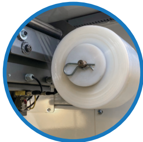
TRAVERSING STRETCH WRAP CARTRIDGE UP TO 21" WIDE.
