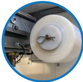
TRAVERSING STRETCH WRAP CARTRIDGE UP TO 21" WIDE.
